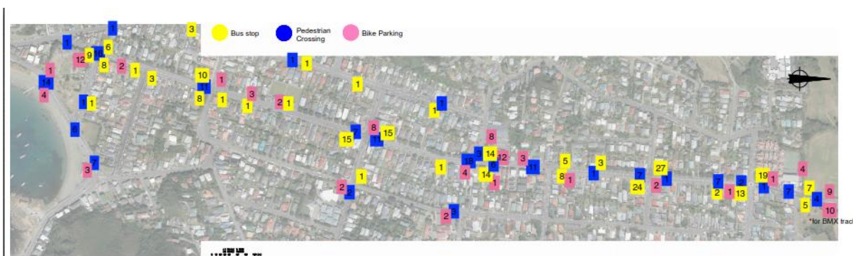
Image showing community preferred bus stop and pedestrian crossing locations along the Parade
