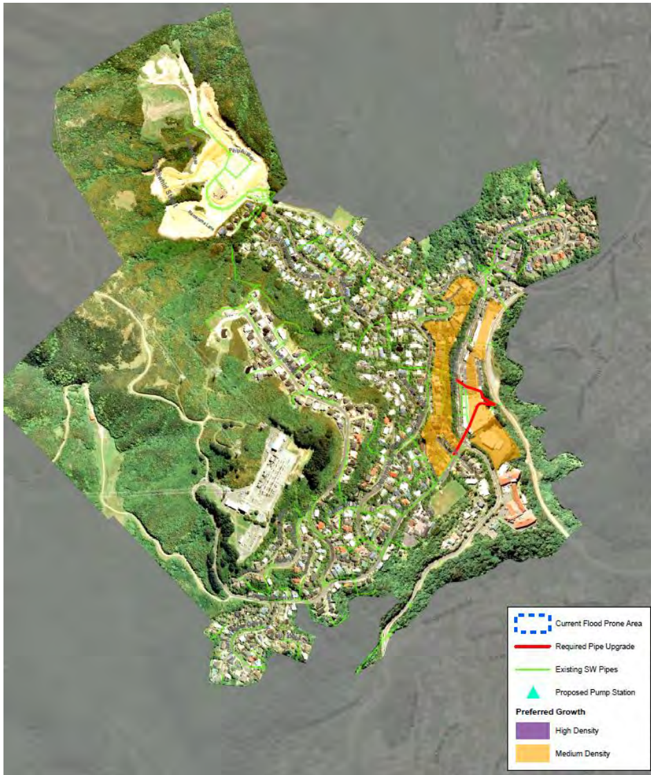
Figure 17 –Potential stormwater upgrades for Crofton Downs
