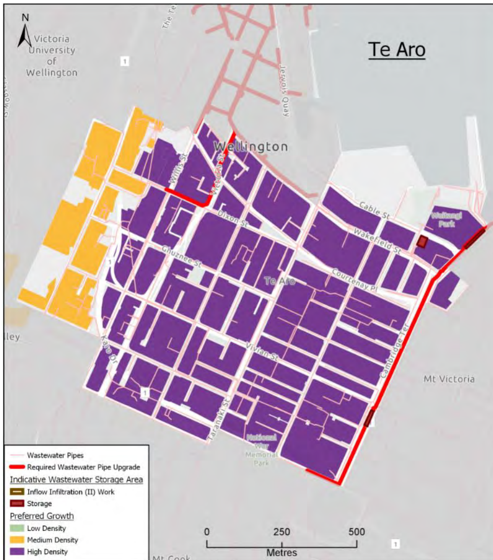
Figure 73 – Proposed wastewater upgrades in Te Aro
