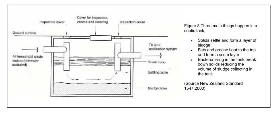
(liquid from the tank) to seep into the soil. In the absorption system bacteria, which occur naturally in the soil, digest septic bacteria and other pathogens so that the liquid is eventually sanitary and does not contaminate the private wells, ponds, or streams. There is some bacterial action in the tank but most of the important action occurs in the soil absorption system. Tanks require periodic cleaning.
