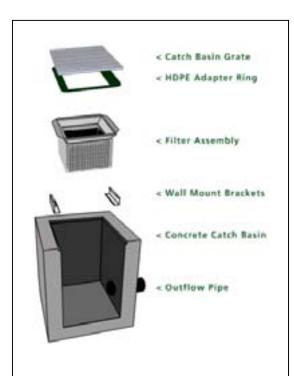
Figure 13 Filter bag set up. Installing such devices would help reduce sediments and chemical contaminants entering the harbour.
