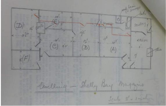
**Fig. 9** Sketch plan showing the Submarine Mining Barracks Building – Caretaker's Quarters in 1925, and the proposed internal alterations to make it suitable for residential purposes. (Item: R21063398, "Defence Works and Buildings – Shelly Bay – Magazine Site," 1926-1953, Archives NZ)
